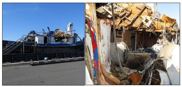
Left, damage to starboard side of the *Specialist's* superstructure after the accident. Right, damage to interior starboard sections of the *Specialist*.
