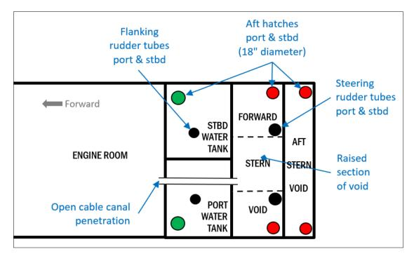
Plan view of *Ricky Robinson* (not drawn to scale). Circles colored red indicate access to void tanks found open with no covers when vessel was salvaged; green indicates hatches for potable water tanks, which had covers in place when vessel was salvaged; and black indicates steering and flanking rudder tubes that passed through voids.
