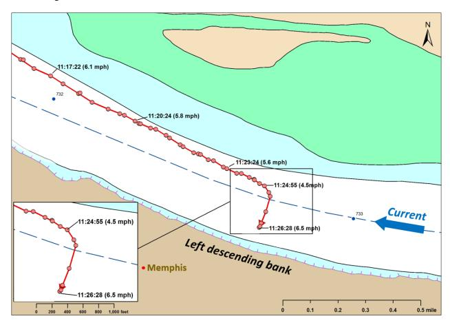
Trackline of *Ricky Robinson*, illustrated with red line, over its last 10 minutes reveals towing vessel's sudden turn to left descending bank just before sinking. (Background from Google Earth)
